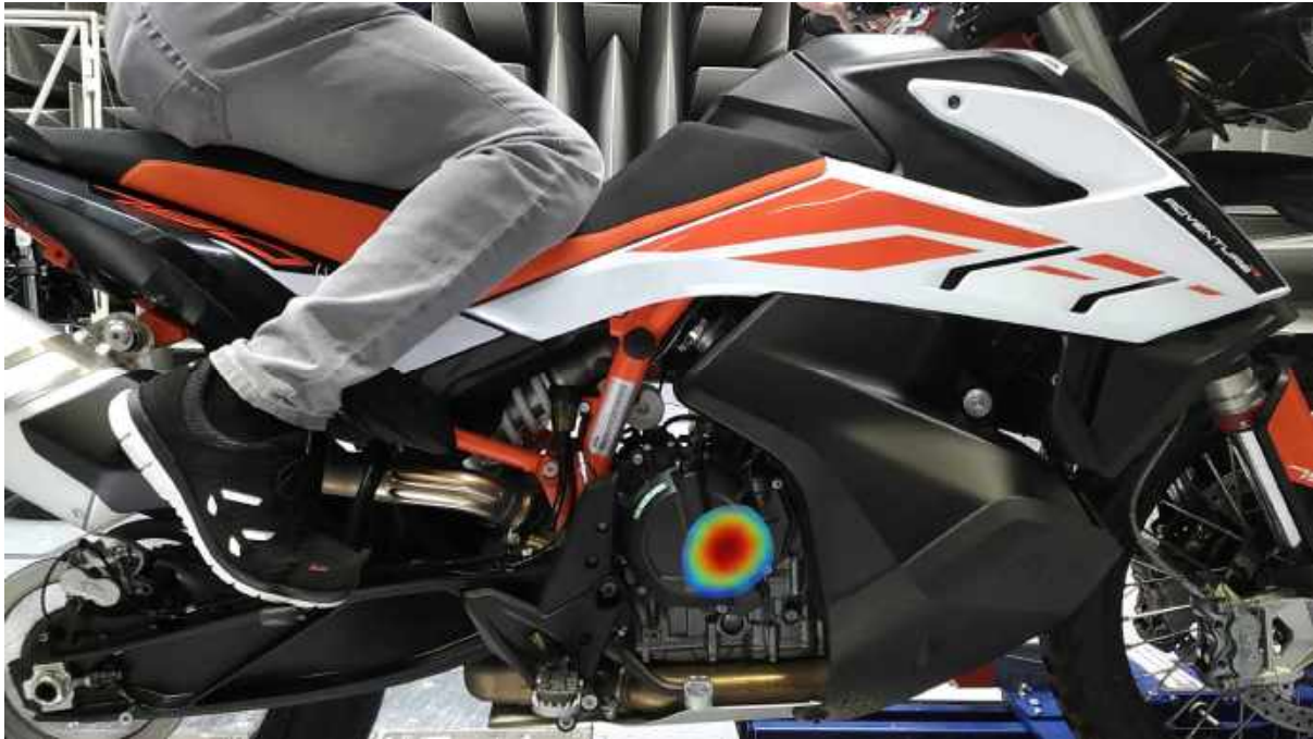
Figure 3 Investigation of surfaces with dominant sound radiation on a roller dynamometer under full load. Acoustic images support engineers during research and development, in adjusting simulation models of engine and transmission components.
